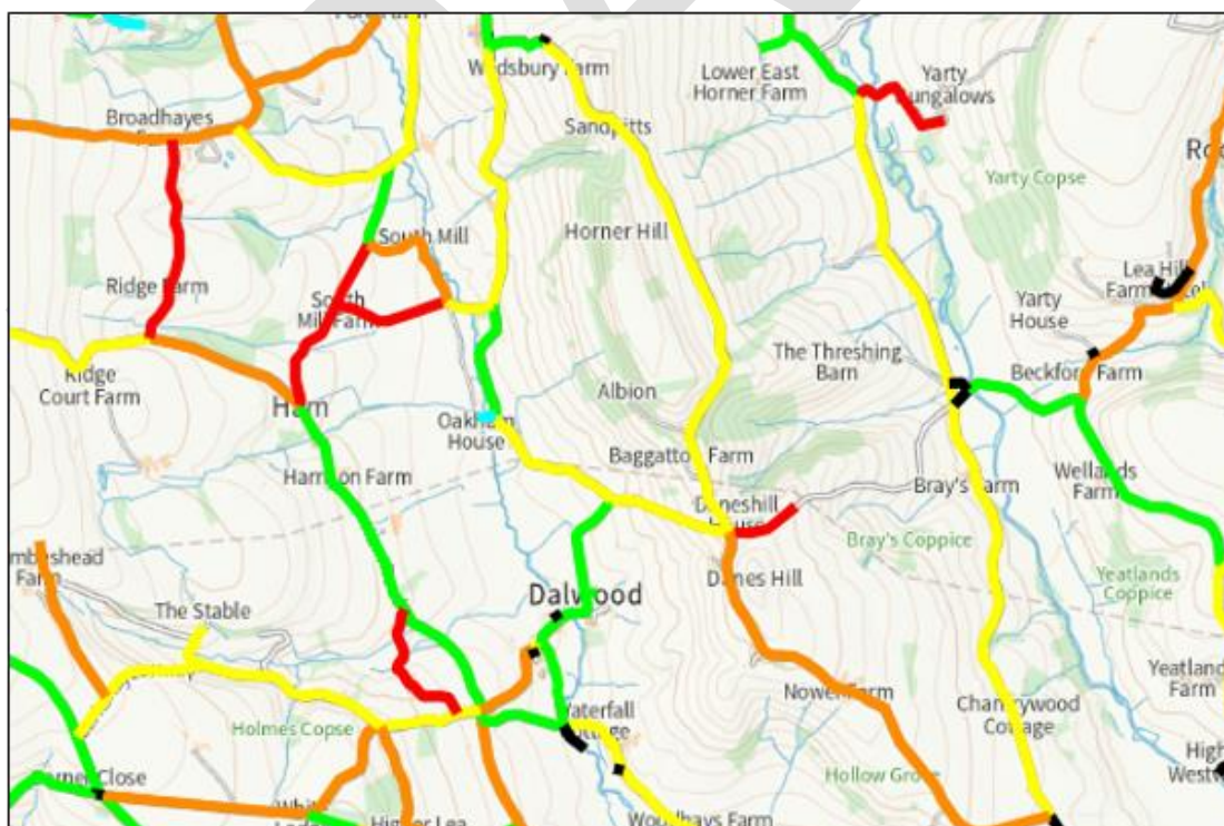
Fig. 1.7: Example of Visual Serviceability Inspection Plan Overlay
